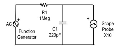
Connect your function generator across the filter and then use the 10x probe and AC coupling to measure the output (middle node) of the filter. Set the function generator to a 5  $V_{pp}$  350 Hz sine wave. Observe the amplitude of the output on the oscilloscope.
