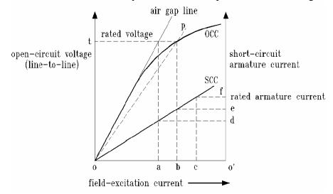
From here you find the rated line-to-line open circuit voltage (point t). From the OCC find the field excitation current that gives the open circuit voltage (point b). Using the SCC find the short circuit armature current that corresponds to the field excitation current (point e). Using the open circuit line-to-line voltage and short circuit armature current the impedance can be calculated as follows:
