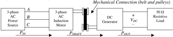
In general a motor is a device that converts electrical energy to mechanical energy and a generator converts mechanical energy to electrical energy.
